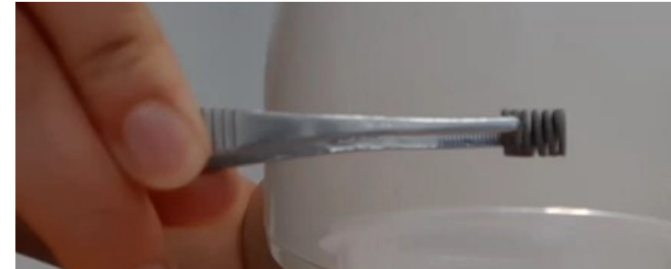
Nitinol 3D printed spring.
