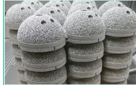
Hip implant produced by Electron-based Powder Bed Fusion 2 (titanium)
