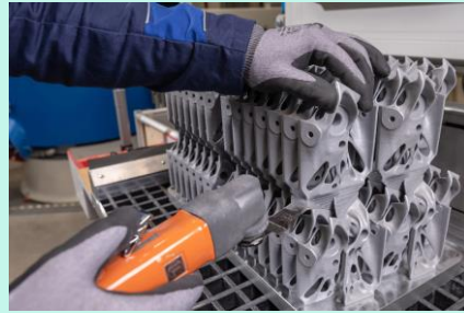
Rolls-Royce body component produced by Laser-based Powder Bed Fusion 1 (aluminium)
