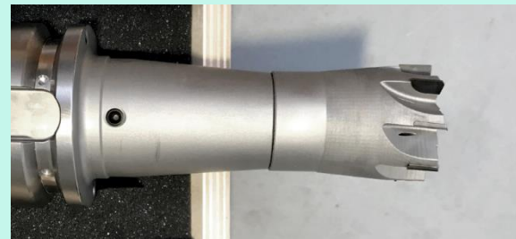
Milling head holder manufactured by means of "Metal-FDM" hybrid 5 (steel)
