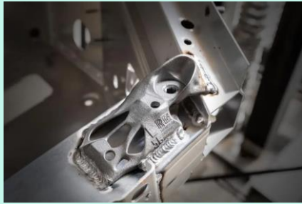
Rolls-Royce body component produced by Laser-based Powder Bed Fusion 1 (aluminium)
