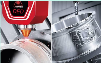
(Large) components produced by (laser) Directed Energy Deposition 3,4 (nickel)
