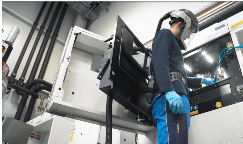
Fig. 4 An operator cleans a machine in preparation for a new build. citim operates twenty-seven AM machines across its sites in Germany and the US
