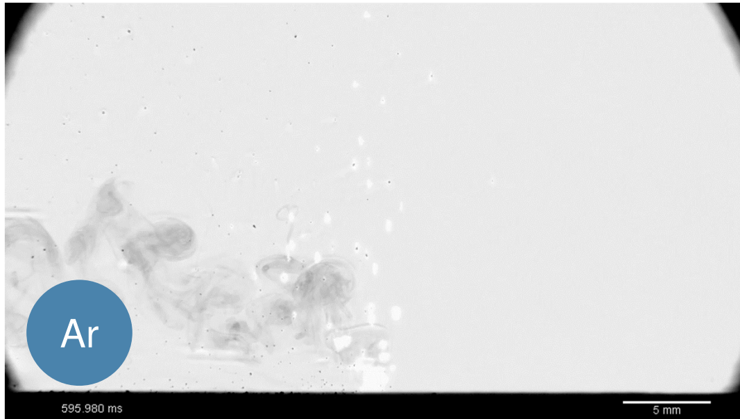
Material: Ti6Al4V, Scan speed: 1,000 mm/s, Layer: 30 \mu m, Specimen: cube Inert gas: Argon (with flow)
